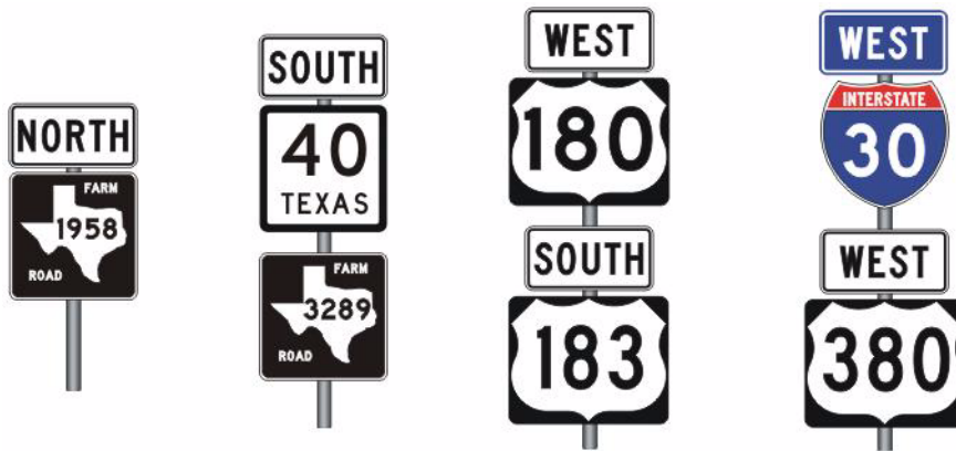
Figure 3-32. Confirming or Reassurance Assembly
