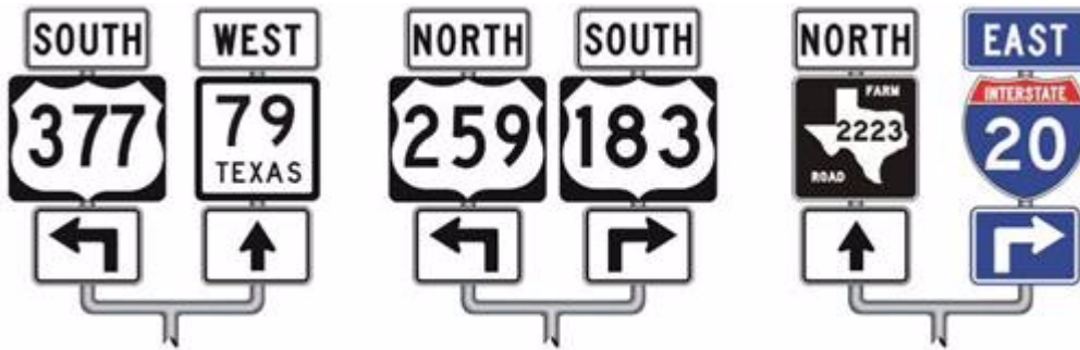
Figure 3-29. Advance Route Turn Sign Assembly
