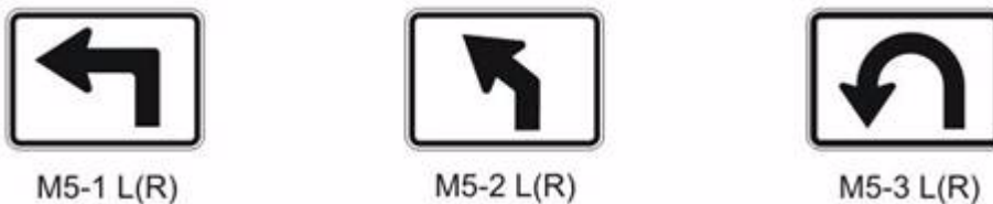
Figure 3-9. Advance Turn Arrow Signs
