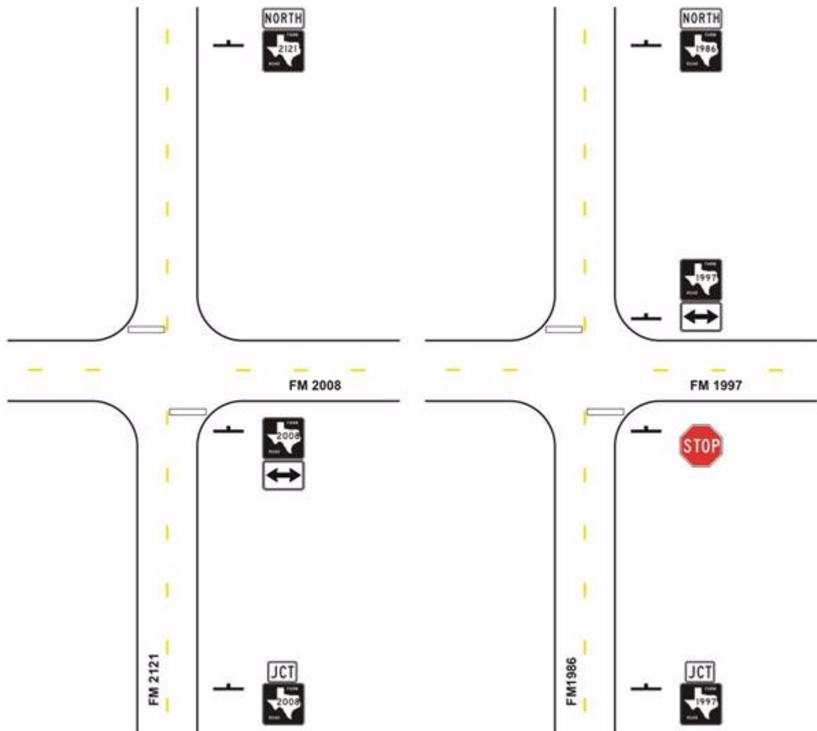
Figure 3-11. Use of Double-Headed Arrow in Directional Assembly
