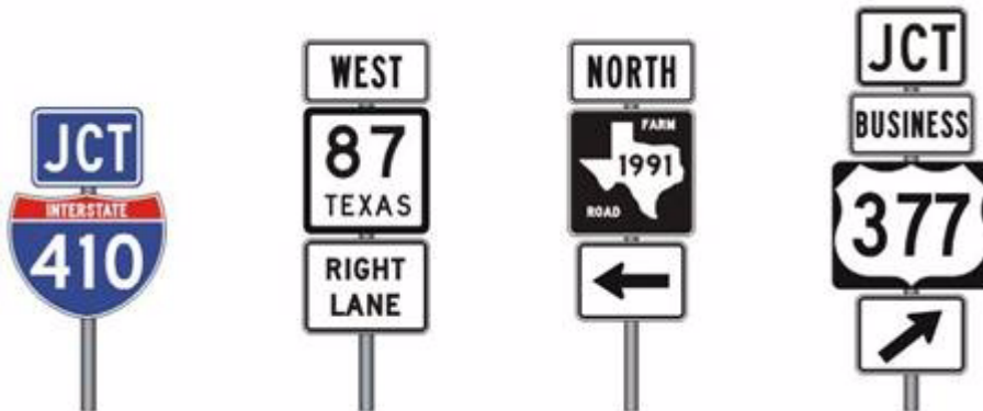
Figure 3-15. Examples of a Guide Sign Unit
